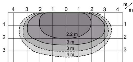
D. LA POSITION DU LOBE EST DETERMINEE PAR L'ANGLE LATERAL DE L'ANTENNE PLANAIRE
