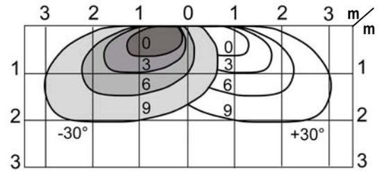
E. LA POSITION DU LOBE EST DETERMINEE PAR L'ANGLE VERTICAL DE L'ANTENNE PLANAIRE
